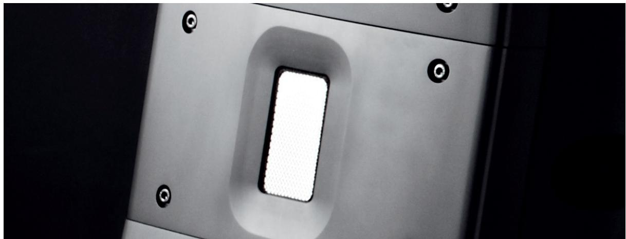
The Raidho Ribbon tweeter FTT75-30-8 is a unique sealed ribbon tweeter. The tweeter employs an array of neodymium magnets to create an extremely powerful force field where an ultra thin membrane is suspended. The membrane weighs less than 0.02 g. Due to low mass the tweeter stores no energy and has no resonances. The performance is extraordinaire and the tweeter leaves absolutely no fingerprint on the speaker system.
