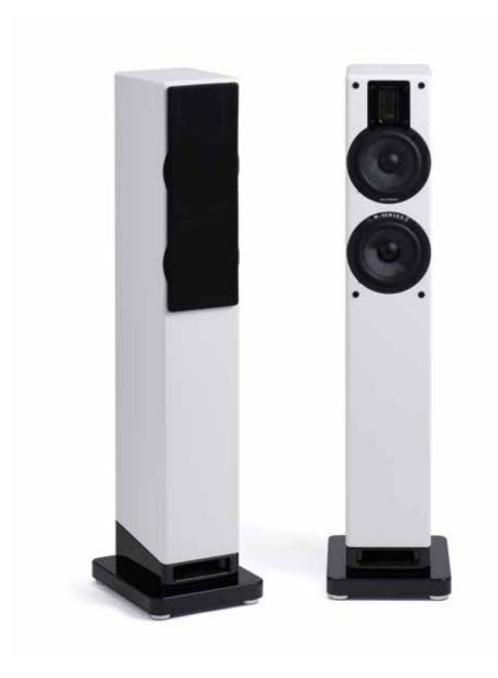
The M-6 is a compact, 2.5-way, floorstanding speaker. The speaker is designed around an ultralight ribbon planar tweeter and two paper-polypropylene compound bass-midrange drivers. The bass driver assists up to app. 300 Hz for added bass capability.
