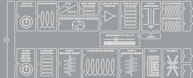
The Mosaic Genesis is a hybridised version of IsoTek's Ultimate series. Combining the extremely low THD sine wave generation engine from Genesis and a lighter version of Super Titan's Direct-Coupled<sup>®</sup> conditioning network, it delivers the perfect balance between power and performance.
