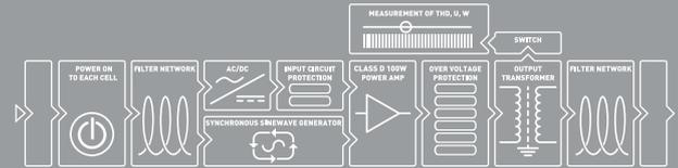
The Genesis One is a state of the art single cell sine wave generation system with extremely low THD. The system can be used to dramatically improve single front-end components. Each cell can be combined / linked together so that only one input wall socket cable is required.
