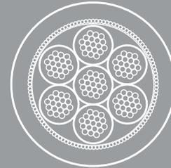
A true high-end cable, IsoTek's Elite uses unique 7-core geometry, high purity copper, and dielectrics to offer astonishing performance. Double shielding with an active OFC braid dramatically reduces RFI and EMI pollution.
