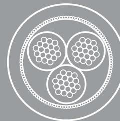
EV03 Sequel refines the multi-strand geometry of Premier as well as incorporating an active shield. The standard fixed length is also increased by half a meter to two meters.
