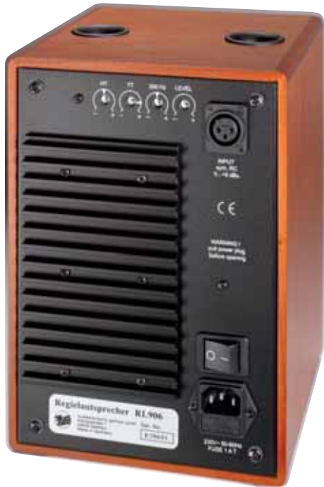
Geithain's filter system has to be adjusted using a screwdriver. As with all studio monitors only a XLR input is provided.
